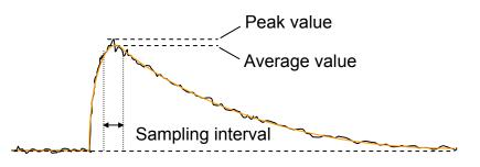
Figure 2: Differences between the peak detector and sample-and-hold circuits.
