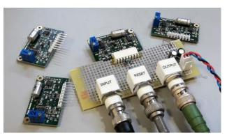
Figure 7: Arrangement used to test the peak detectors. Two 10  $\mu$ F electrolytics decouple the power rails while a 470  $\Omega$  resistor and a small Zener protect the reset input from overzealous pulse generator settings.
