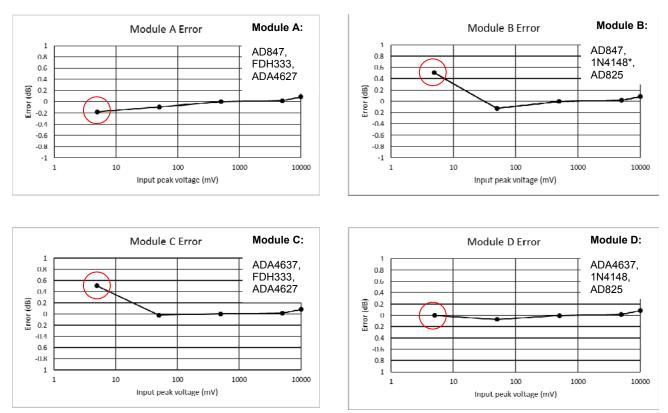
Figure 15: Amplitude response of the four versions of the circuit using a continuous 5 kHz sinewave input. The circled readings should be taken with a large pinch of salt and depend on input offset adjustment; see text for explanations.
