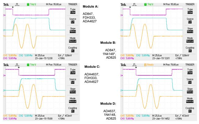
Figure 9: Response of the four versions of the circuit to 20 V peak-peak two cycle sine burst at 20 kHz. The reset signal (pink) takes the circuit out of reset just before the input burst (yellow); output is the blue trace (\* = SM).
