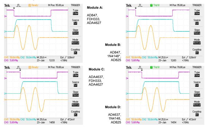
Figure 11: Response of the four versions of the circuit to 200 mV peak-peak two cycle sine burst at 20 kHz (\* = surface mount).
