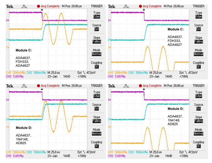
Figure 17: Performance of the clamping circuits for modules C (top) and D (bottom). The clamp circuit performs equally well for both positive and negative DC input voltages.
