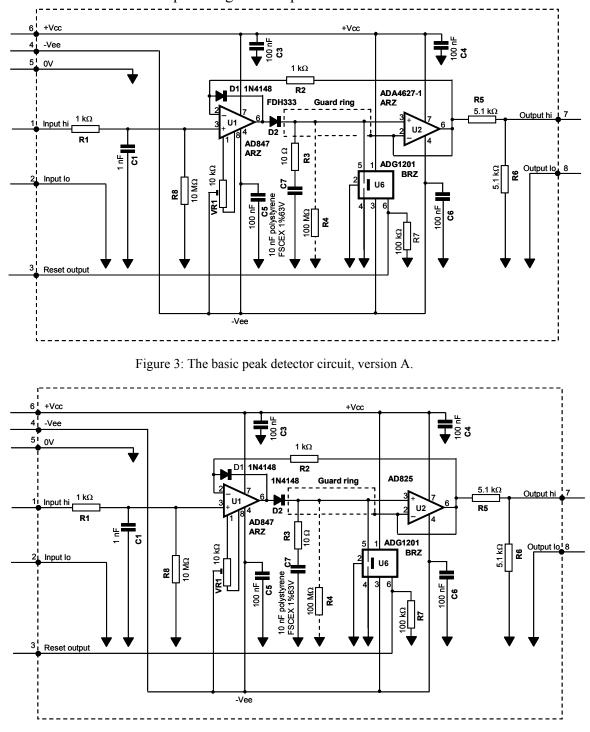
Figure 4: The basic peak detector circuit, version B.
