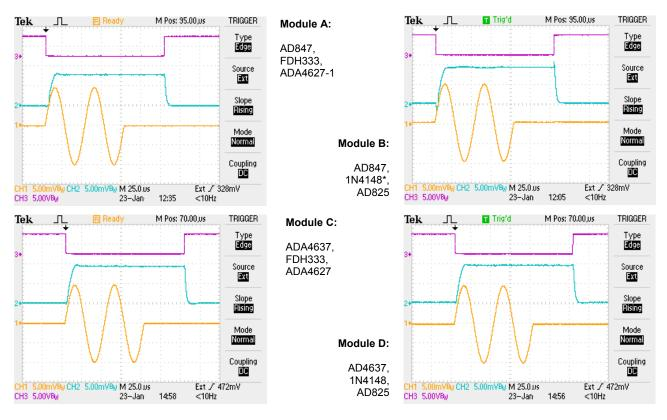
Figure 12: Response of the four versions of the circuit to 20 mV peak-peak two cycle sine burst at 20 kHz (\* = surface mount).
