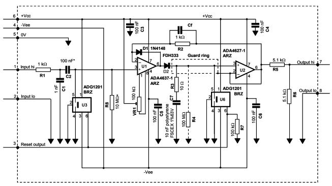
Figure 5: Circuit of peak detector circuit with input clamp. Version C. Capacitor Cf, empirically determined to be 150 pF, was soldered across R2: helps tame this particular opamp combination.
