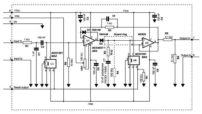
Figure 6: Circuit of peak detector circuit with input clamp. Version D. Capacitor Cf, empirically determined to be 150 pF, was soldered across R2; helps tame this particular chip combination.
