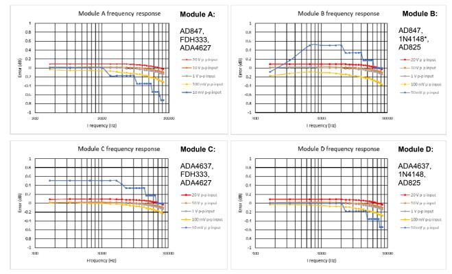
Figure 16: Frequency/amplitude response of the four versions of the circuit at different input levels (continuous sine wave input); (\* = surface mount).
