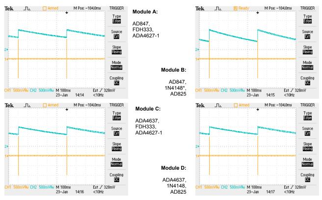
Figure 13: Droop performance of the circuit versions following sine monocycles at 2 Hz; discharge resistor R4 in place (\* = surface mount).
