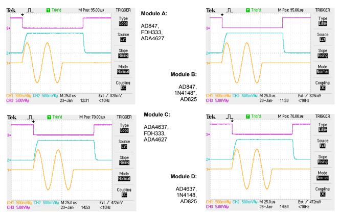
Figure 10: Response of the four versions of the circuit to 2 V peak-peak two cycle sine burst at 20 kHz. Trace colours as in Figure 9.
